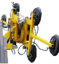
The **Automotive** suction unit was developed for operating at the GML. It is supplied with energy by the lift and is suited ideally for overhead glazing, 90°tiltable by remote control. The frame can be extended by 6 to 8 suction plates.
