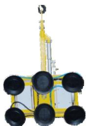
The **Bus suction unit** with swimming stored suction plates is ideal for the sure admission and exact assembly of curved glass.
